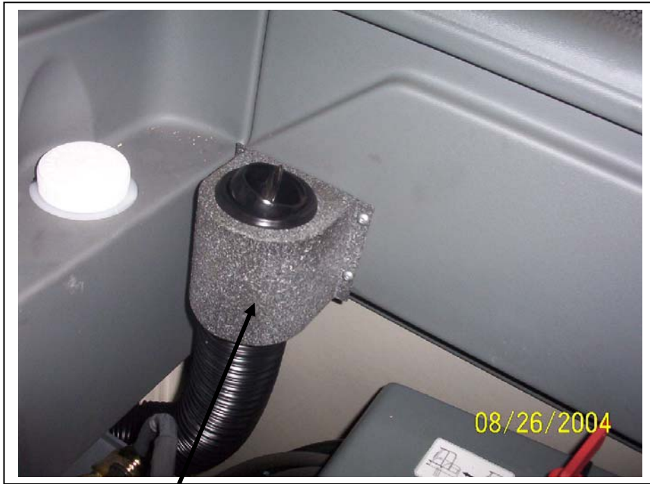
Extra louver installed in the back left corner of the cab. Use the self drilling screws provided. Connect the flex hose to the louver before mounting.
