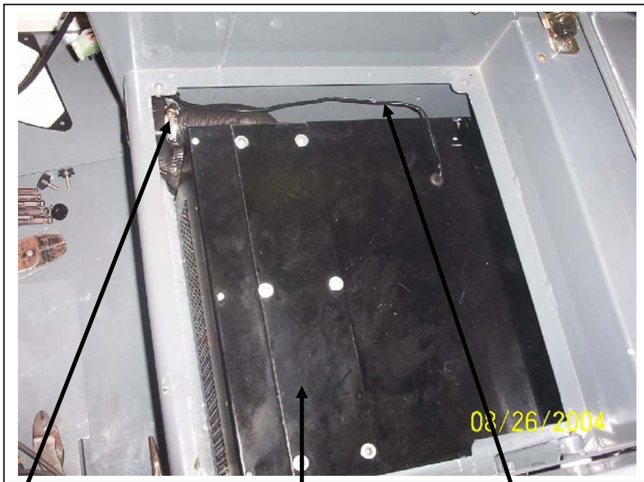
Louver and flex hose back in place
